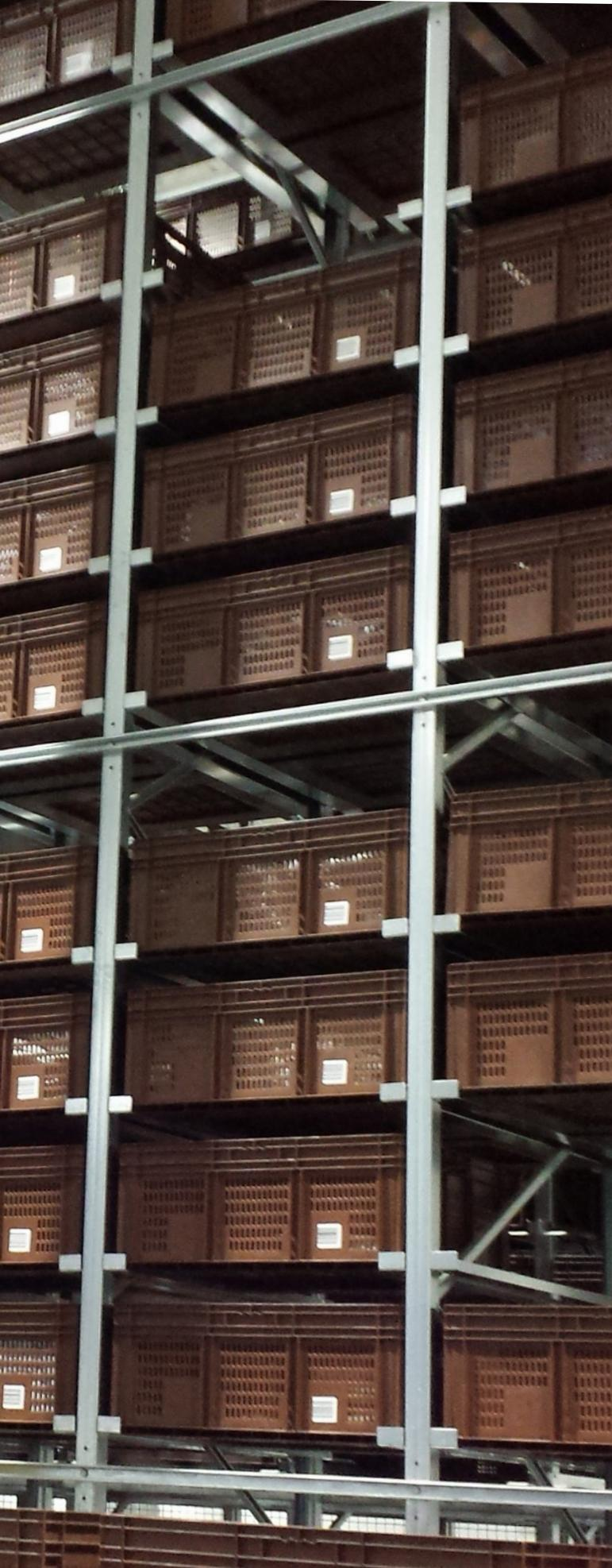
Mini-load Automated Storage and Retrieval Systems (AS/RSs) are also often used for small parts or eaches. Two aisles of narrowly spaced racking comprise Mini-Load AS/RSs. A Storage and Retrieval Machine (SRM) moves between the aisles in two dimensions, at rates of up to 100 cases per hour per aisle (use depending). These systems typically handle items smaller than 100 lbs.
