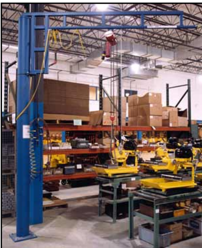
Work Station Jib Crane
