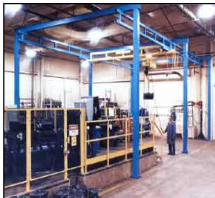
Work Station Bridge Crane
